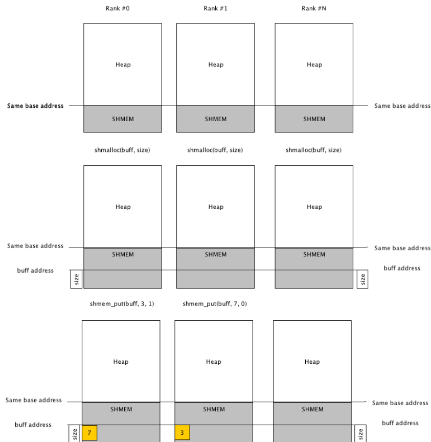
Figure 3 Memory layout of a SHMEM program. Notice that the Symmetric Heap (SHMEM in the figure) has the same starting base address in all ranks. When a symmetric allocation routine is called in all PEs, the heap grows symmetrically. Since the pointer to buff is the same, put/get routines can put data using the same address in all ranks.
